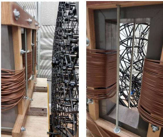
Fig. 5. Testing arrangement of acoustic camera and scaled electrical transformer.
