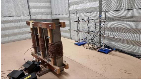
Fig. 3. Conventional nine microphone array test arrangement placed 70cm from the transformer.
